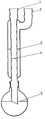
Fig. 1. The modified apparatus: 1,2 - ground joints, 3 - level of cooling liquid, 4 - level of the cooled part of the reaction mixture, 5 - level of the heated part of the reaction mixture.
